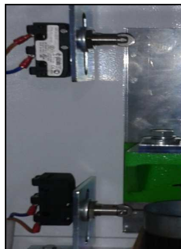
BMR20 bowl lifting micro-switch
