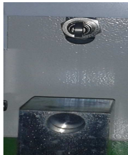
BMR20 bowl lifting micro-switch
