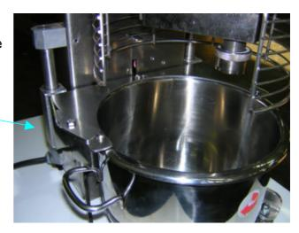
8.3) Rotate the bowl guard in the open position, select the appropriate tool and insert it onto the tool shaft. Insert the tool clockwise so that the notch on the agitator fits over the pin on the tool shaft as shown in the picture.
