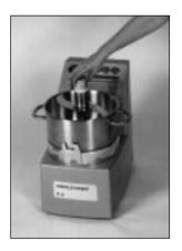
3) Position the blade mounted on the motor shaft. Then rotate it so that it is lowered right down to the bottom of the bowl.
