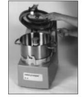
5) Close the lid by pressing the front of the lid. Continue applying pressure, fasten the catch to the front of the bowl and lower
